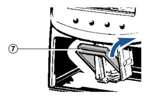
Dirt and dried up ink at the holder of the ink cartridge can be removed with a soft cleaning cloth moistened in spirit (see figure1)
